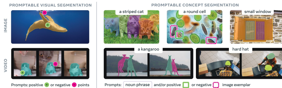
Figure 15.56: Promptable visual segmentation vs. promptable concept segmentation in SAM 3. The left side illustrates promptable visual segmentation (PVS), where SAM and SAM 2 segment a single object per prompt using clicks, boxes, or masks. The right side shows SAM 3’s promptable concept segmentation (PCS), which segments all instances of a concept specified by a short noun phrase, image exemplars, or their combination. Figure reproduced from [65].
