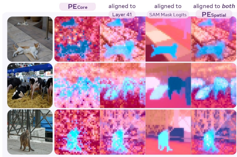
Figure 15.62: Final-layer PE feature visualizations (PCA to LCh). PE Core (second column) captures semantics but exhibits noisy, spatially incoherent patterns. Distillation to an intermediate PE layer (third column) restores coarse spatial coherence but boundaries remain fuzzy. Distillation only to SAM 2.1 logits (fourth column) produces sharp boundaries but inconsistent semantics across similar objects. The final PE Spatial model (fifth column) combines both: sharp edges with semantically consistent regions, ideal for dense concept segmentation and tracking. Figure taken from [48].
