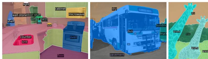
Figure 14.41: Panoptic segmentation with DeTR-R101. DETR can segment both “things” (object instances) and “stuff” (amorphous background regions) in a unified manner. The consistency and alignment of masks show that DETR learns strong spatial and semantic priors. Adapted from [64].
