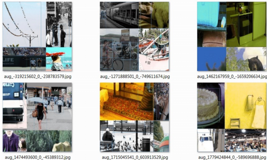
Figure 13.22: Mosaic augmentation in YOLOv4. Source: [47]. Four input images are stitched into a 2 \times 2 grid, allowing object instances to appear in unfamiliar contexts and at smaller scales. Unlike CutMix, which blends only two images, Mosaic mixes four scenes simultaneously, encouraging robustness to background variation and spatial layout. Notably, this design enables BatchNorm to compute statistics over four different images per batch, reducing the need for large batch sizes.
