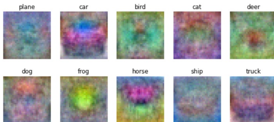
Figure 3.8: The output of the code (building upon NumPy and Matplotlib) visualizes the rows of the weight matrix reshaped into the input image format, enabling inspection of the learned templates.
